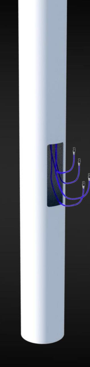
Untie (cut all zip ties) all cable works and drop them through the middle of the pole. Make sure they all can be reached at the mast service door. Check the functionality of the cables.
