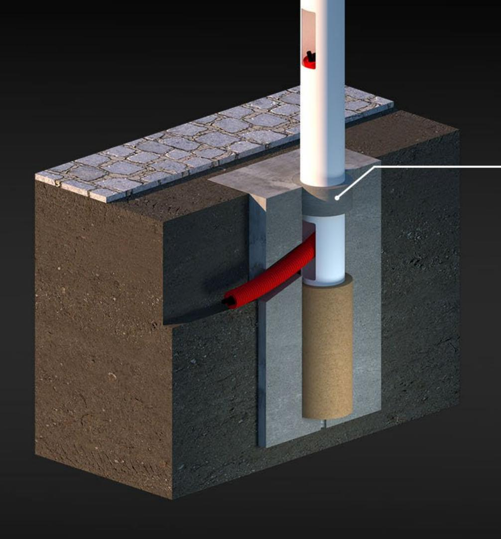
Secure the construction with fine concrete cap
