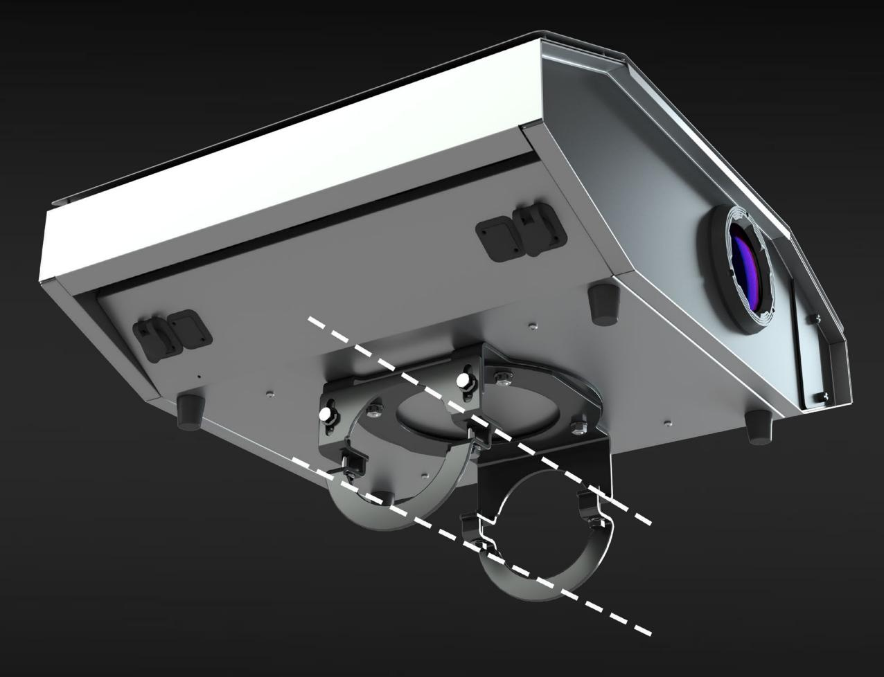
Place the projector on top of the X-part connector. Aim the lens towards the illuminated surface. Use the black Circle Plate and bolts to secure the projector in position.
