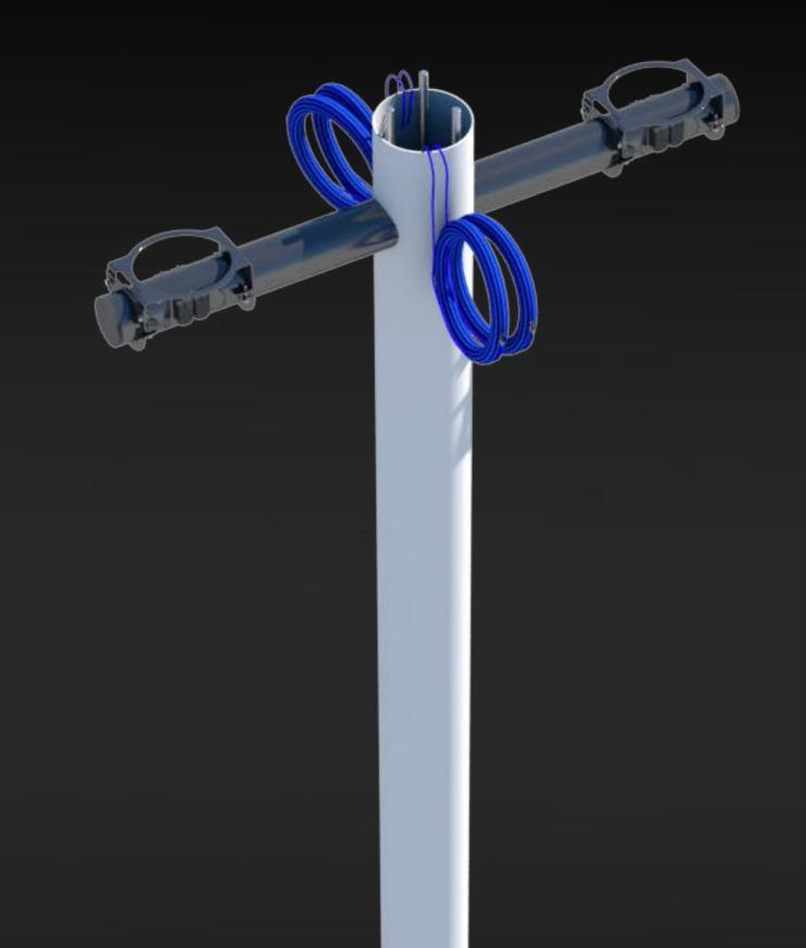
Use Projector Identification and Alpha Angles from the Project Specific Documentation you printed earlier. Put the X-part on the urban mast connector according to the Alpha Angle. Make sure that the Powercon and LAN connectors face backwards from the projection screen.
