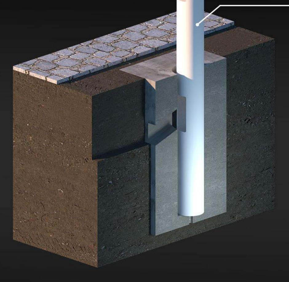
Secure the post in perfectly vertical position with wooden pieces. Make sure the door is accessible for the underground cable insert.
